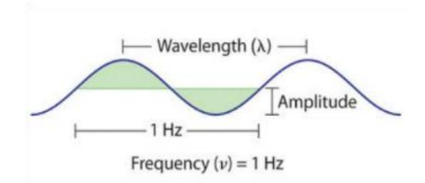
**AMPLITUDE** – one half the height of a wave (intensity)
